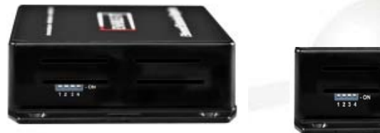
Default DIP settings 860 CPE – All down set in the ON position 860 CO – DIP position 1 up (OFF) DIPs 2-4 down (ON)
